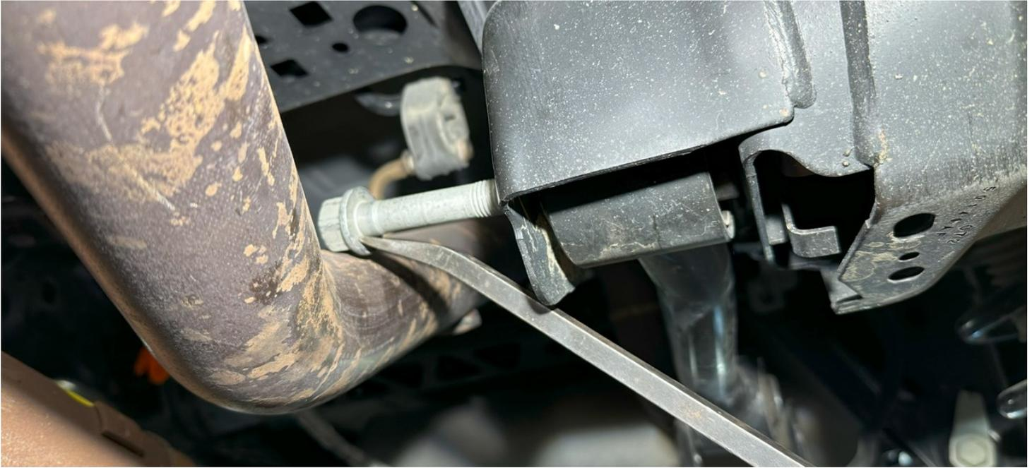
15. Also on driver side — With the arms removed, trim the “tang” on the lower, axle side bolt to 1” to ensure it doesn’t contact the Carli Arms when reinstalled.
