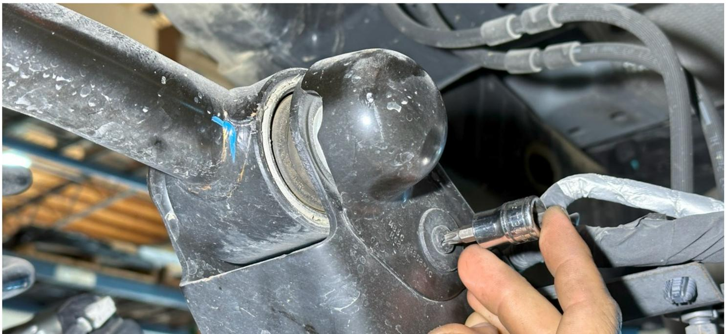
10. **T25 Torx** — Remove the bolt cover from the frame mount.
