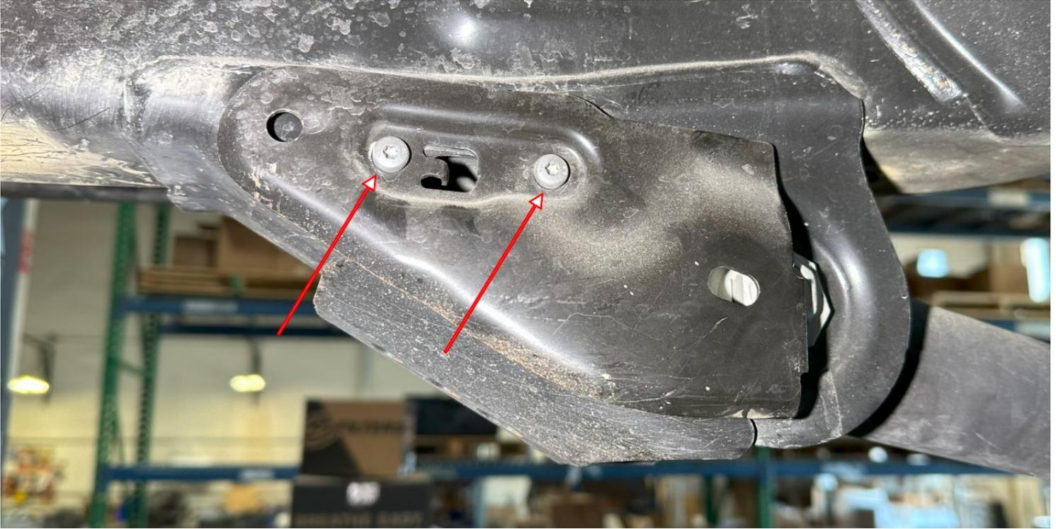
11. **24MM** — NOTE ALL BOLT ORIENTATIONS (the factory hardware will be used install the Carli Arms), support the axle with jack stands and remove both upper and lower factory control arms on the Passenger side. ONLY work on one side at a time — this, with the track bar, will ensure the axle stays put while you're swapping the arms.
