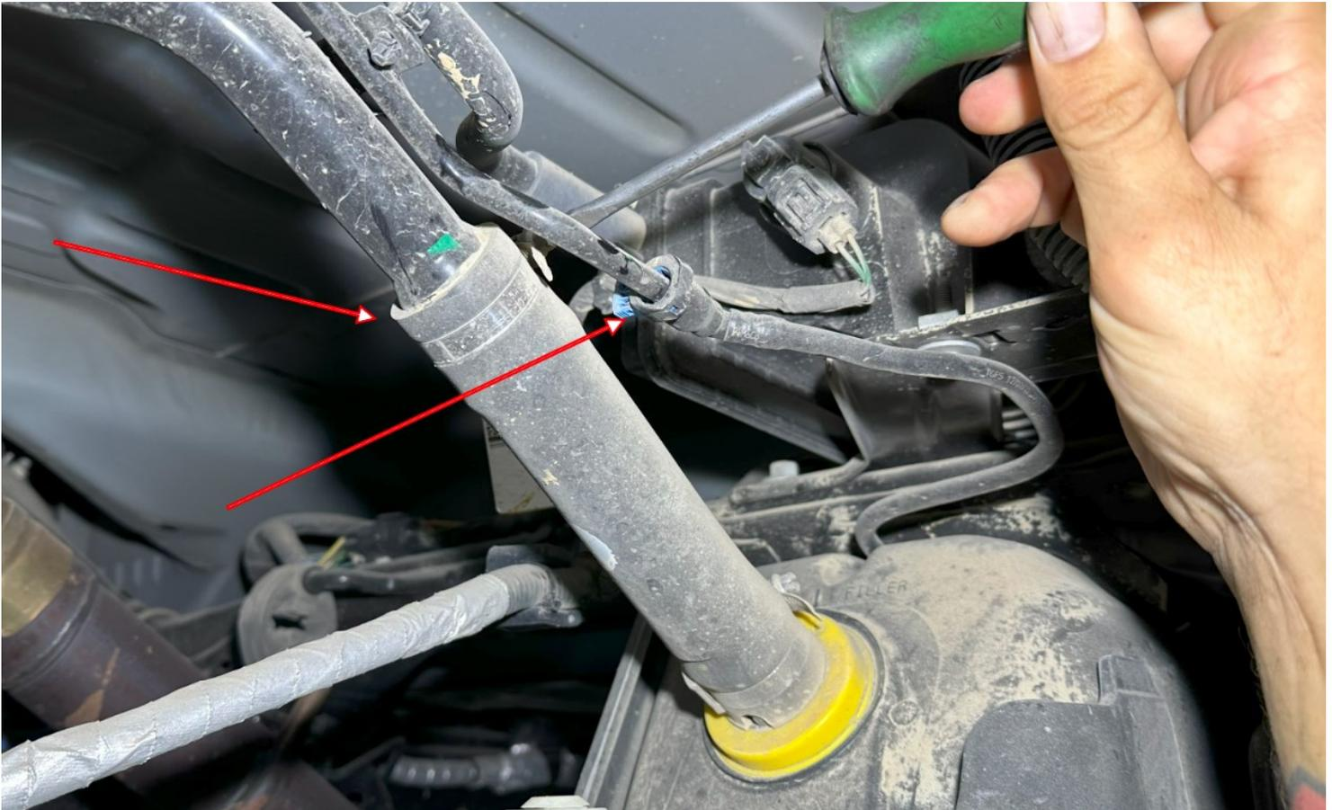
5. Disconnect the two fuel line connections at the front of the tank.
